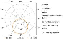
13,8 W Yes, STEINEL LED system LED cannot be replaced 1550 lm 3000 K
